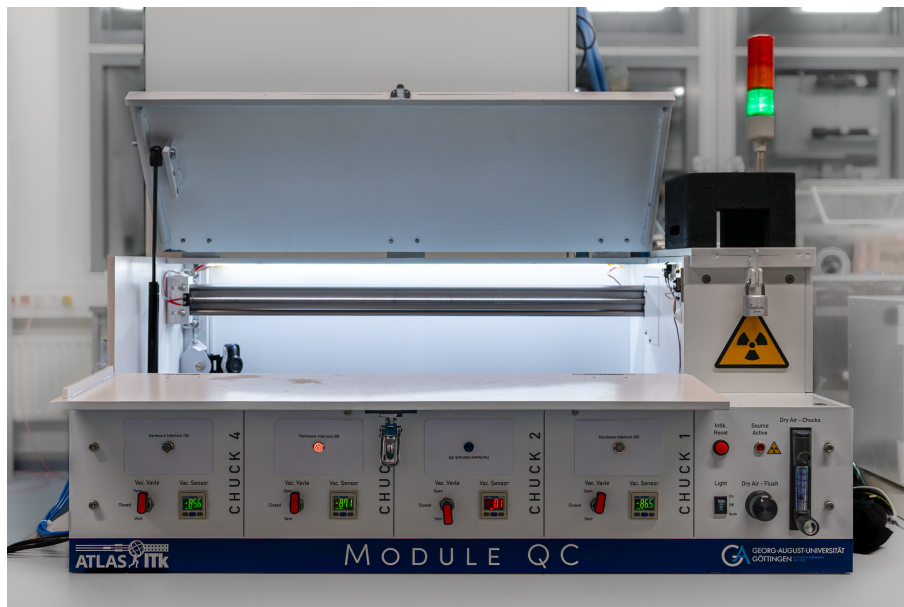
Figure 8.1.: Electrical testing setup for the ITk module production in Göttingen, constructed as part of this thesis.
