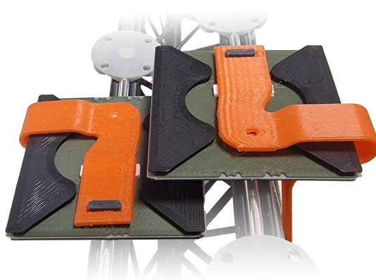
Figure 4.6.: Physical model showing the positioning of Outer Barrel Modules on an LLS, including folded pigtail (orange) and OBWBP (black).
